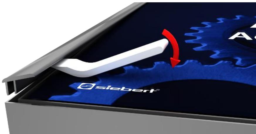
Open the device by using the lever tool. First remove the connectors and then the front pane. Upon delivery, the connectors are only applied loosely.
