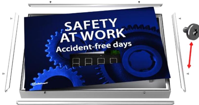
To open the device remove the torx screws and keep them carefully for later assembly.
